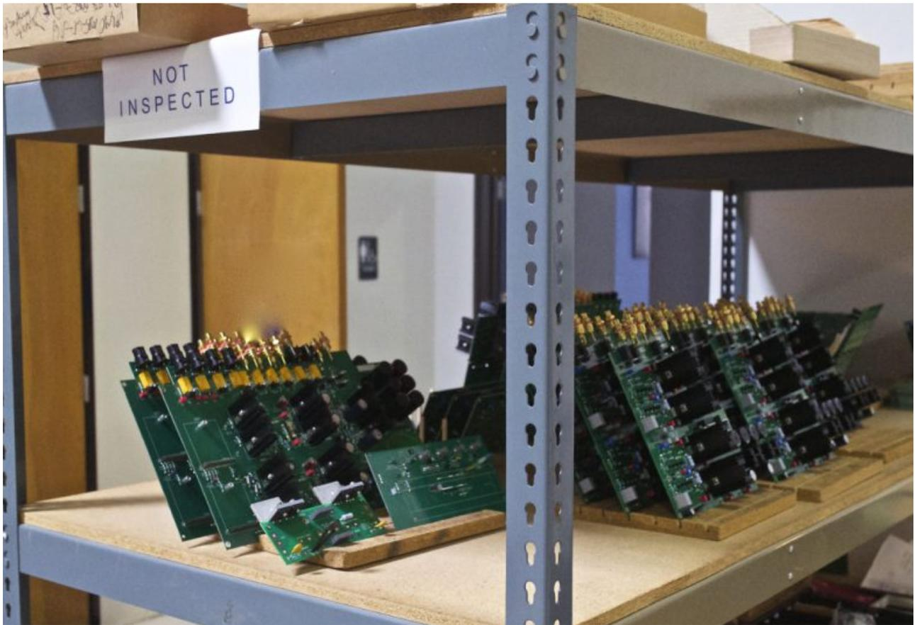
After assembly, the circuit boards are moved to a shelf with an incredibly fancy sign, well at least a sign that is easy to understand. There they sit to await inspection by a technician.
