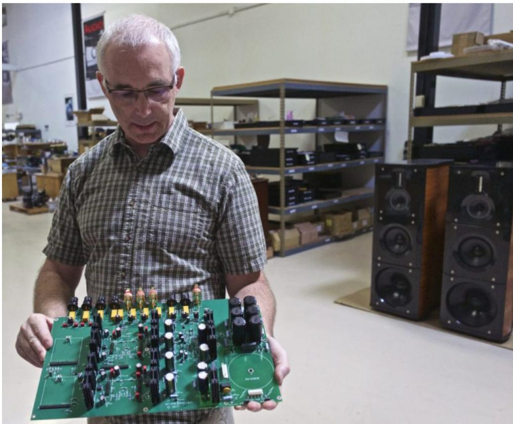
Desmond began the tour by showing us a circuit board before it had been through inspection. These are assembled there at Pass Labs by hand.
