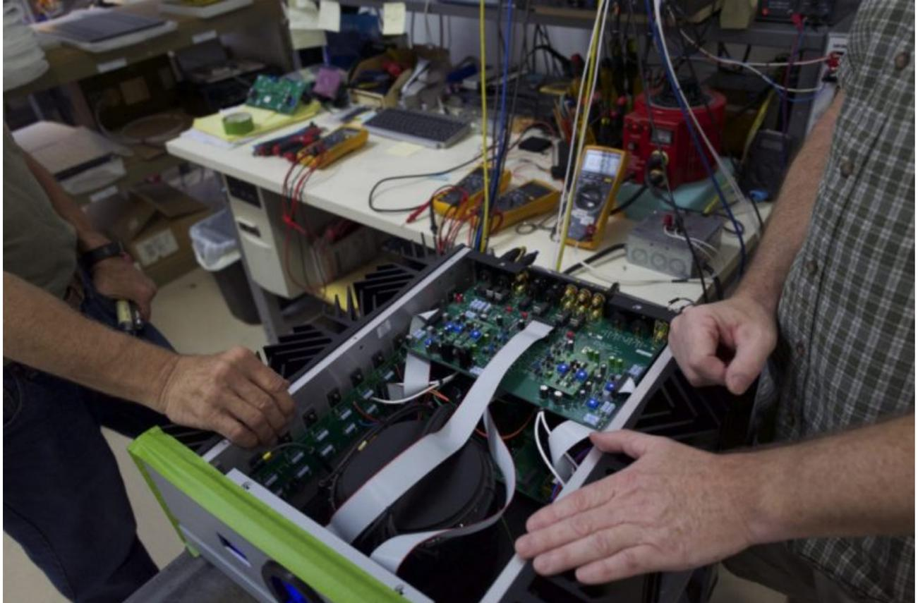
After the amps and preamps are assembled, they are taken to a room that is kept at the same temperature year around for break-in and biasing. This assures that the bias of every Pass amp that goes out is identical. All Pass amps are burned in by running power through them for three days.
